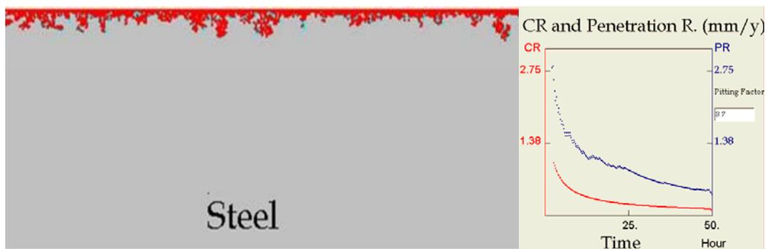
Figure 4.12 Film morphology and corresponding corrosion rate predicted by 2-D model at 0.54bar  $p_{CO_2}$ , 30ppm  $Fe^{2+}$ , 80 °C, pH 6.6, 1m/s
