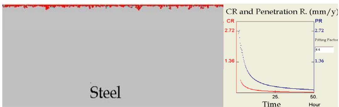
Figure 4.13 Film morphology and corresponding corrosion rate predicted by 2-D model at 0.54bar  $p_{CO_2}$ , 50ppm  $Fe^{2+}$ , 80 °C, pH 6.6, 1m/s
