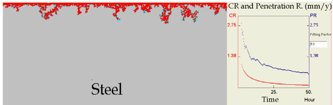
Figure 4.11 Film morphology and corresponding corrosion rate predicted by 2-D model at 0.54bar  $p_{CO_2}$ , 28ppm  $Fe^{2+}$ , 80 °C, pH 6.6, 1m/s
